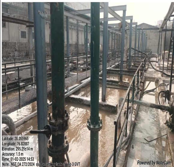
Sludge settling tank installed of unit-I, II&III separately for treatment of waste water and treated water recirculated through flow meter in the process with PTZ camera to check ZLD
